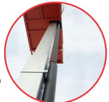
The revolutionary mast lifting system designed by BRAVI PLATFORMS for all its platforms models represent a real change on its sector! The mast made of a special extruded aluminium is 100% maintenance free! No more chains to be regularly inspected, no more grease or lubricant required, no maintenance: a real low cost ownership!
