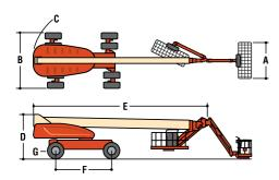
**Standard Features** Platform: 36 x 96 in. (0.91 x 2.44 m) Side Entry 8 ft (2.44 m) JibPLUS° Boom Selectable Capacity Envelope 180° Hydraulic Platform Rotator AC Receptacle in the Platform 5 Degree Tilt Alarm/Indicator Light All Motion Alarm Swing-Out Engine Tray 12V DC Auxiliary Power Hourmeter Control ADE® System Full-time 4WD 3 Selectable Steering Modes Drive-out Extendible Axles Oscillating Axle **Proportional Controls** Gull-Wing Hoods
