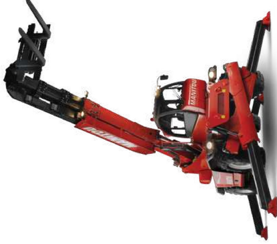
Rotation on lowered stabilizers with 1500 kg jib
